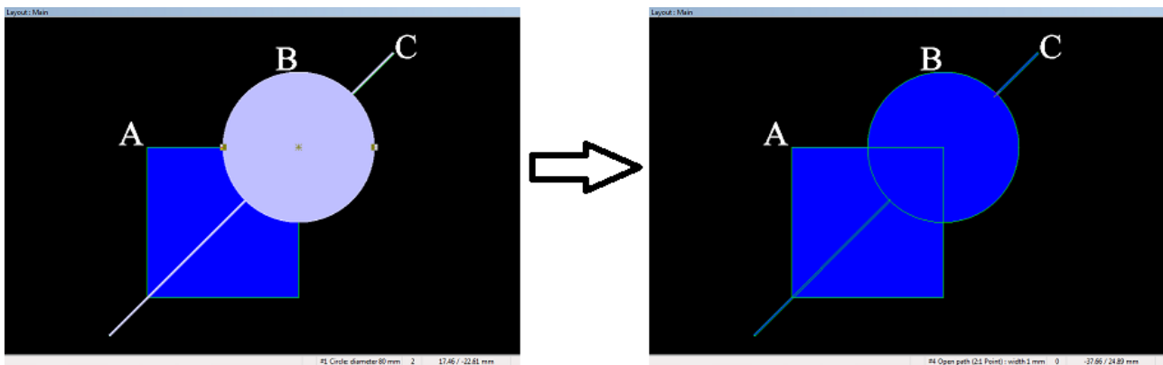
Figure 200. After the two objects B and C are selected, the Paths off Area operation is executed, the result is trimming of the path C as shown
