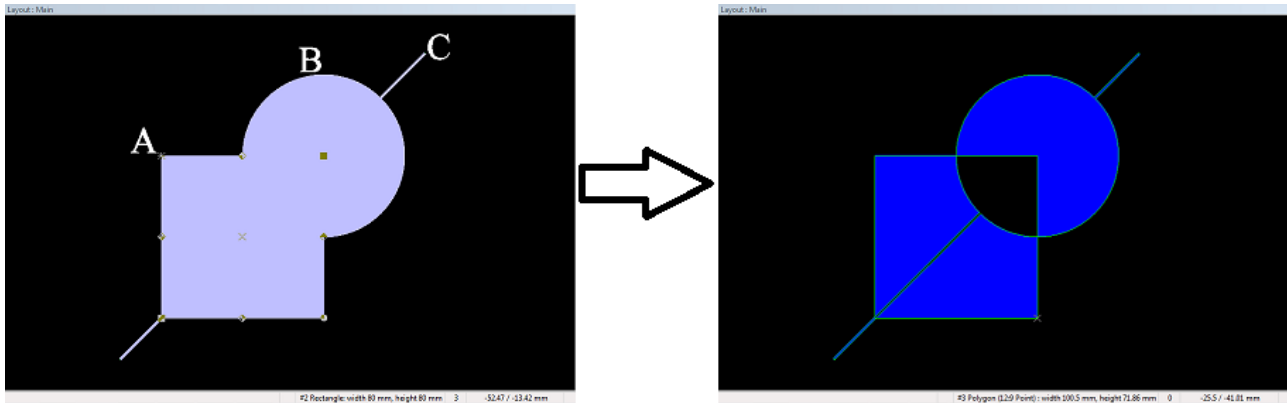
Figure 195. After the three objects A, B, and C are selected, A is the primary selected object (operator); the XOR operation is executed, the result is a set of new polygons
