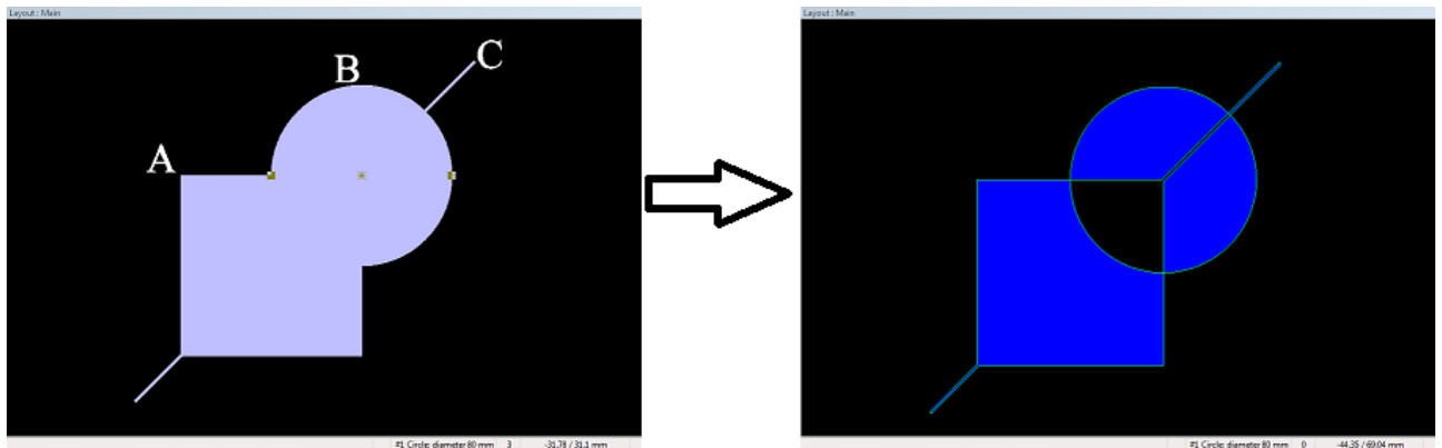
Figure 196. After the three objects A, B, and C are selected, B is the primary selected object (operator); the XOR operation is executed, the result is a set of new polygons
