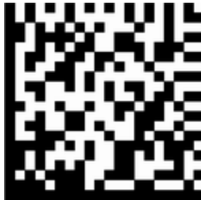
Figure 362. Example of Data Matrix code, encoding text "Always a cut ahead"
