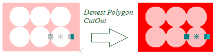
Figure 175. Denest Polygon CutOut initial data (selected one hole) and result (denested all holes)
