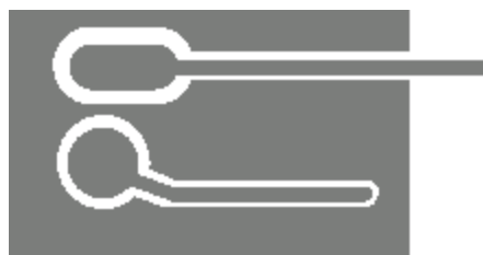
Figure 360. Result of copper pouring
