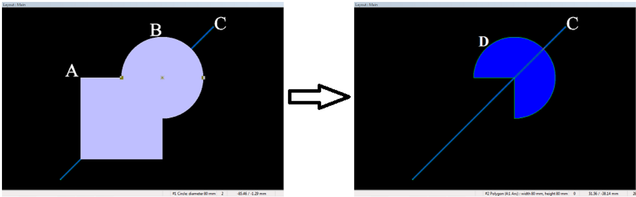
Figure 189. After the two objects A and B are selected, B is the primary selected object (operator); the difference operation is executed, the result is a new polygon D
